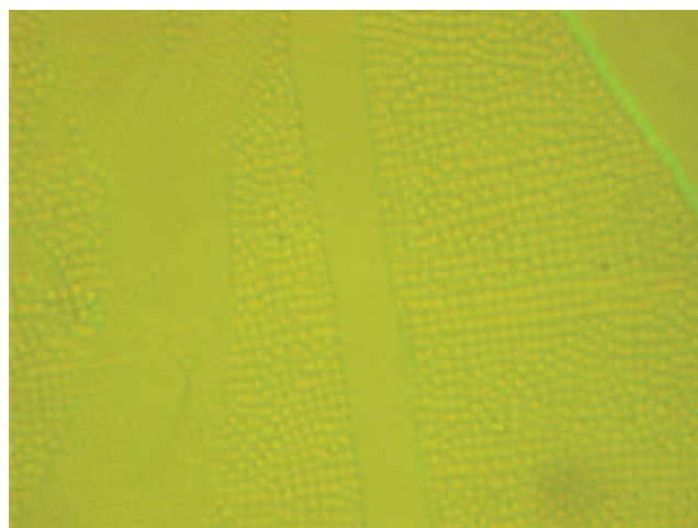
Figure 2. UV-induced structural changes, ‘crocodile skin’ structure..
